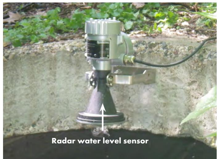
Figure 2: Radar water level sensor
