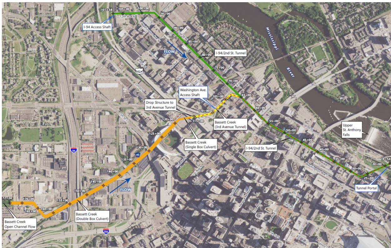
Figure 1-1 Tunnel System Overview
