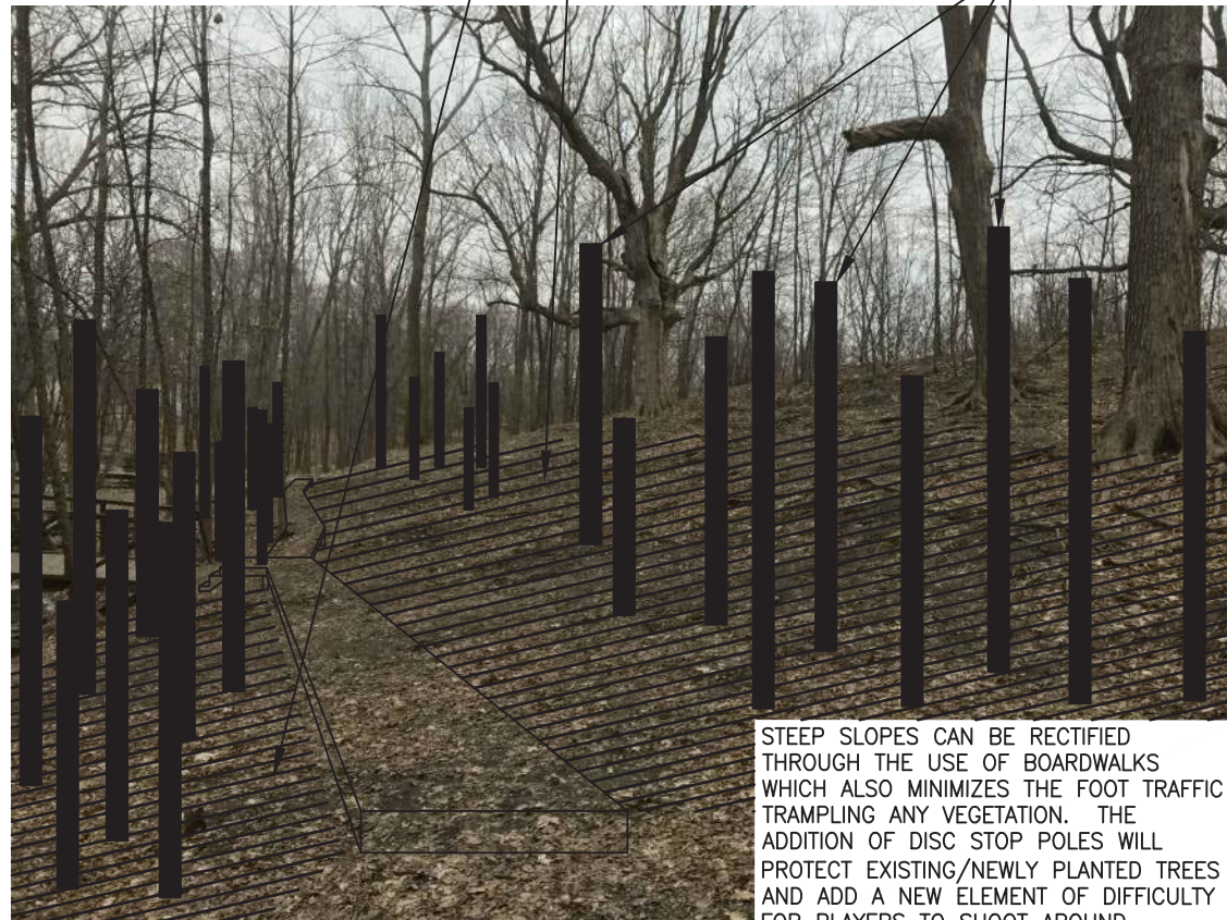
EXISTING TREES WITHIN THE FLIGHT PATH ARE SCARRED BY DISCS REPEATEDLY HITTING THE SOFT TISSUE OF YOUNG TREES. TO PROTECT THE TREES DISC STOP POLES WOULD BE PLACED BETWEEN THE TREE AND THE DIRECTION OF FLYING DISCS. WITH STAGGERED ROWS OF POLES DEFLECTION WILL SERVE TO PROTECT TREES.
